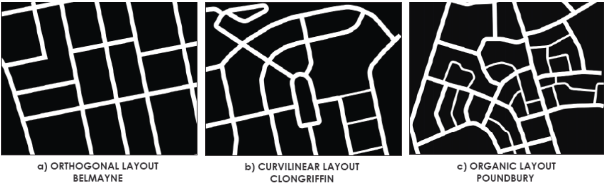
Figure 6 | Permeable Street layouts (Source: Figure 3.8 – DMURS)
